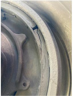
• 10/3, at the White River inspection site, Inspector placed a dump truck out of service for a leaking air reservoir tank due to a defective weld. The truck had no State of Vermont inspection, and the carrier was issued a Vermont Civil Violation Complaint.
