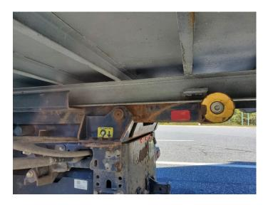
• 10/3, I91 SB Rest Area Hartford, Inspector conducted a Level 1 inspection on a TT unit and found that the airline to axle #2 drivers side brake had chaffed through the outer protective layer and the reinforcement ply. The vehicle was placed OOS until the violation was repaired.
