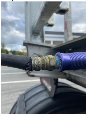
• 10/01 – Insp. inspected a tractor trailer combination at the US Rte. 4 Fair Haven scale house detail. The inspection revealed a brake hose was improperly joined, and electrical wiring was in contact with the exhaust system. The truck tractor was placed out of service.
