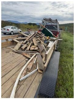
• 9/24 – Cpl. inspected a tractor trailer unit at the US Rte. 4 Ira rest area detail. The inspection revealed the load was secured improperly as belly straps were needed on the second tier of the wood products. The driver added strap(s) and remedied the out of service defect.
