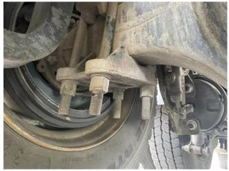
• 09/24 Coventry detail, Inspector conducted an inspection on an interstate commercial motor vehicle whose driver was under the age of 21. It was also discovered 20% of the brakes in use were defective due to a push rod not connected to a slack adjuster and was out of adjustment. The driver and vehicle were placed out of service.
