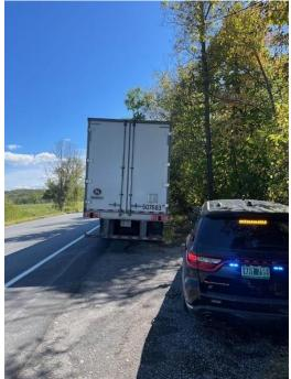
• 9/23--Insp stopped a combination tractor/trailer for a load securement issue on I89 in Randolph. An inspection was conducted, and the trailer was placed out of service for inoperative turn signals and a defective brake hose.
