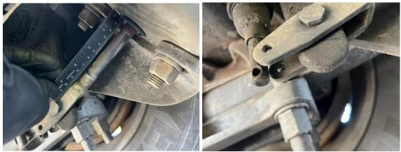
• 9/26, Cpl. inspected an interstate combination and found multiple brake air hose violations, including a massive air leak on a chafed service brake air hose and two improperly spliced brake hoses, which resulted in the vehicle failing to maintain air pressure. The vehicle was placed out of service while in combination for the improperly spliced air connections, chafed air hose and failure to maintain air pressure.
