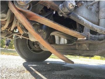
• On 10/16 Rte. 7 Leicester VT, Inspector conducted a level 1 inspection and located an axle positioning part that was broke causing the axle to shift. In the photo you can see at the top the broken mounting plate for the axle positioning part and the gap between the axle and the spring pack, also there was a cracked frame supporting the fifth wheel.
