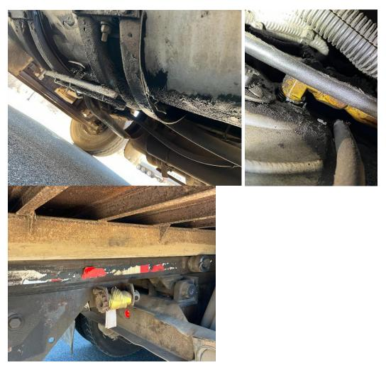
• 11/13, Guilford, An Insp. discovered a brake out of adjustment on a 2-axle box truck; the slack adjuster had not compensated for wear and the brake accounted for 25% defective brakes. Additionally, three box/frame mounting bolts were found to be loose. The truck was placed out of service for brakes and repaired roadside.
