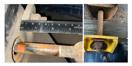
• 11/13, Guilford, An Insp conducting a Level 1 inspection on a box truck, found a loose body mount on the front passenger side of the box.
