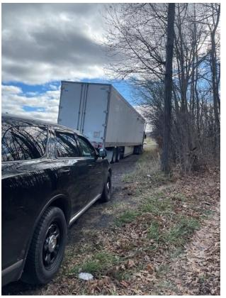
• 11/19, Inspector stopped a truck hauling an excavator on Route 4 in Woodstock. The machine weighed over 10,000 pounds yet the boom was not secured to the deck. The truck had a non-manufactured hole in the brake can. The truck and trailer were placed out of service.
