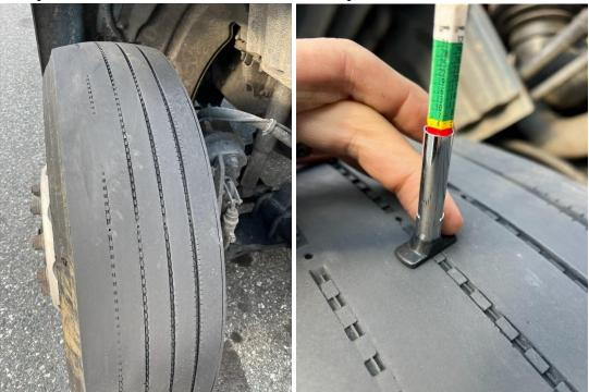
• 11/19, Hartford, Cpl. discovered a reservoir air tank with broken flanges securing the tank to the trailer, as well as three trailer brakes out of adjustment and a dual set tire with less than 1/32". Although the air reservoir tank movement did not meet the out of service criteria, the combination was placed out of service for greater than 20% defective brakes.
