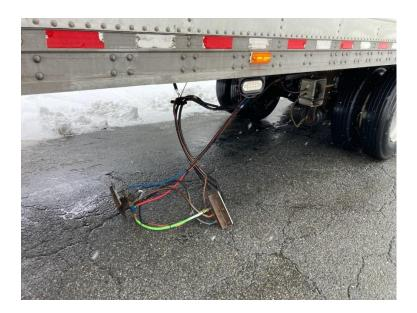
• 12/5, Springfield, Cpl. discovered an improper emergency breakaway cable attachment on an interstate combination vehicle. Additionally, a defective tiedown was found with a two-inch cut on a sharp edge, an excavator was secured using only 5 tiedowns when 6 were required, and a flat tire on the trailer. The trailer was placed out of service until the defects were corrected.
