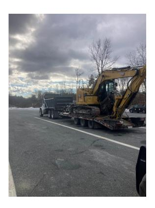
• 12/3, at the White River Detail, Inspector placed a trailer out of service for improper load securement. The front bucket was not secured to the trailer deck of a machine weighing over 10,000 pounds.
