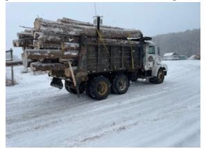
• 01/30 Fairlee, Inspector conducted an inspection on a commercial motor vehicle in commerce with no USDOT numbers displayed. It was discovered the carrier had no USDOT numbers, the driver was not medically certified, and the breakaway was not attached to the power unit. These were first offense violations, and the driver was educated for what was needed for interstate commerce and repaired the breakaway violation on scene.
