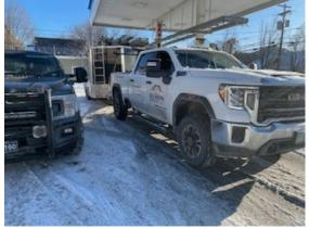
• 01/30 Wells River, Inspector conducted a traffic stop on a commercial motor vehicle for an unsecured excavator weighing more than 10,000 lbs. The excavator only had two tiedowns securing the load when required four and the accessory equipment was unsecured. Inspector conducted an inspection of the vehicle and was subsequently placed out of service.
