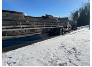
• 01/29 Berlin, Inspector conducted an inspection on a commercial motor vehicle and discovered the breakaway was insufficient and unable to be attached to the power unit and 3 of 4 tires on the trailer were flat. The vehicle was placed out of service.
