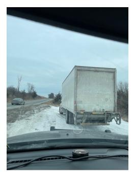
• 1/28-Insp stopped a tractor trailer on I-89 in Randolph for a dimension violation. An inspection was conducted, and the trailer was placed out of service for a projecting load greater than 48inches with no flag/s as required. The driver was educated and issued a warning.
