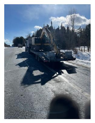
• 1/28- Insp stopped a commercial motor vehicle driveaway/towaway for a marking violation and the rear light bar had become detached from the vehicle and was hanging on the ground. An inspection was conducted, and the vehicle was placed out of service. The driver was issued a warning.
